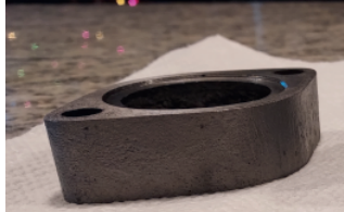
Above: Original spacer off my dad's car. Notice the rough outer surface. This would not be recreated on the new part.
