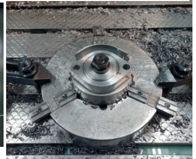
Below-right: Spacer after milling and drilling was completed. Still in the mill.
