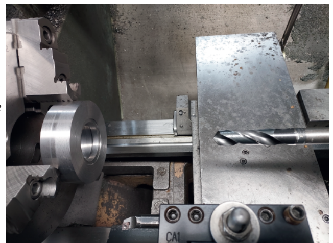
The slug of steel in the lathe once drilling and boring were completed
