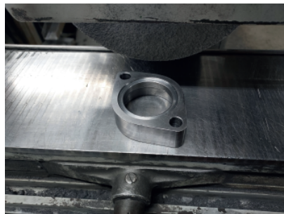
Above: spacer bolted back into the lathe showing the "extra material" that needed to be removed after milling.
