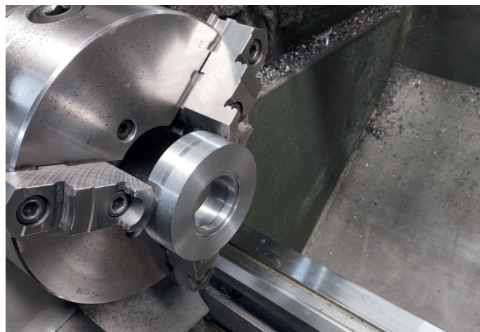
The slug of steel in the lathe once drilling and boring were completed
